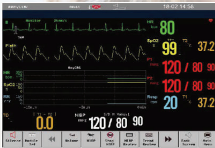
Other bed Display other bedside monitor's all parameter and one waveform, support user defined parameter display
