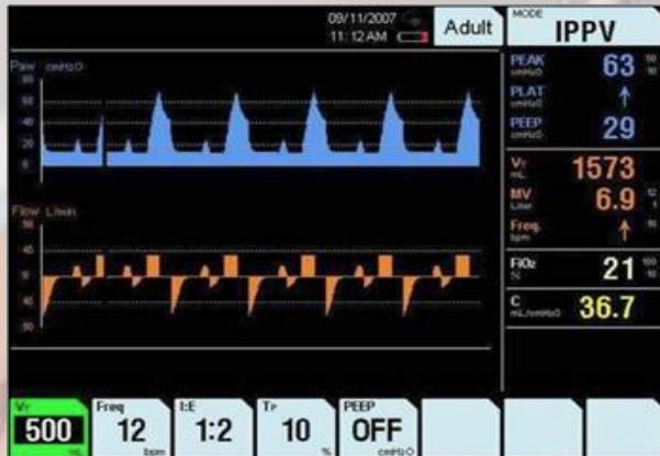
The parameter monitor is in the left and right side of the user interface, the wave form in the middle. When there is a menu popping up, the wave area will be covered. The upper section is message area, the middle section is monitor area, the under is parameter area.
