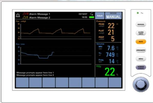
The anesthetic ventilator not only provides patients in operation with auto ventilation, but also monitors and displays the patient's various parameters. The anesthetic ventilator used in the system is controlled by microprocessor, and it configures monitor internally, volume mode, and other functions. The ventilation parameter monitor, setup and message notice of the ventilator are all displayed in the user interface.
